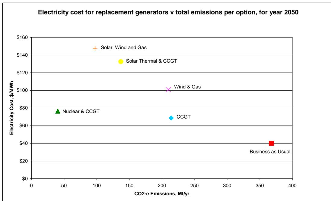
**Figure 12:** Long run marginal cost of electricity (\$/MWh) in 2050 (for the coal and replacement technologies only) versus total emissions (t CO<sub>2</sub>-e/MWh) from all the technologies in each option.
